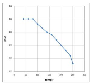
\*Max. Temp. 260° F (126.7° C) 230 psig Unit can be used to 20° F (–6.7° C) @ 400 psig
